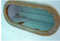
Next I removed the old boxes, took some measurements and constructed the boxes. I gave them a few coats of oil based enamel. The next task was to figure out how to attach them. I decided to “glass” some small angle brackets to the inside of the fiberglass. This involved a lot of climbing into the cockpit locker to enter the cavity under the cockpit seats. Good thing I’m
