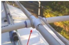
apart. Middle fitting is a "cross", only glued from the sides. I run an old sheet from the back arch to the front arch, snug and tie it to keep the frame together
