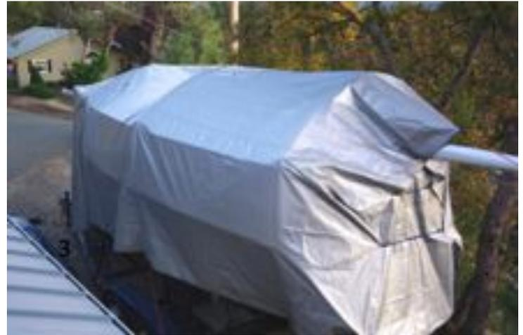
to cover the end of the boat, cutting a hole in it to slip it over the mast, then draping that piece over the back arch. The main tarp goes on and I close the back in with bungees. I have to do it this way because the next size tarp is way too big. This keeps the boat very dry all winter. To make this, you need: PVC glue and primer, About 60' of 1" PVC Pipe, 6 - 1" 45 degree elbows, 2 - 1" Tees, and 1 - 1" Cross "T." Total should be no more than \$20-\$25 to make the arches.
